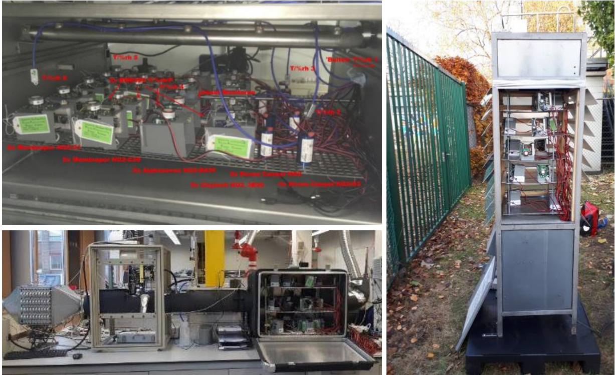
Figure 4: Sensors within the exposure boxes in the laboratory (left) and within the shelter at the field site (right).
